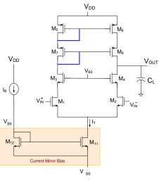
**Problem 5** Assume the amplifier in Problem 4 is designed so that the excess bias of all transistors is 300mV,  $V_{DD}=1.8\text{V}$ ,  $V_{SS}=-1.8\text{V}$ , and the power dissipation is 25uW,
